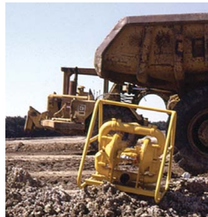
Construction Dewatering Pump
