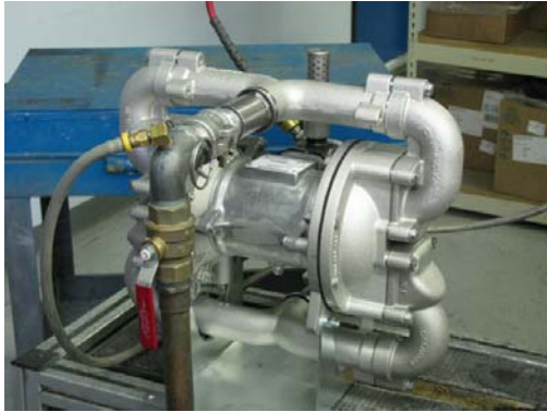
Tank recirculation/Transfer Pump
